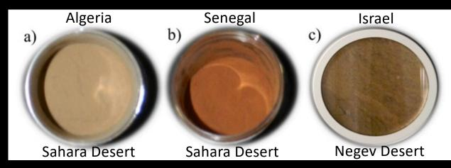
Soil samples from desert regions taken for the Fennec field campaign and the Statistical Evaluation of Aerosol Retrievals (STEAR) experiment. The different hues illustrate the high variability of mineral composition of dust sources.
