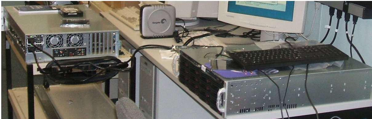
Figure: Two Core i7 workstations interconnected via 10 Gigabit Ethernet in test configuration prior to shipping to SC09.
